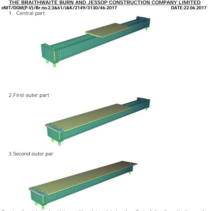
Construction joints should be positioned to minimize the effect of the discontinuity on the durability, structural integrity and appearance of the structure. Joints should be located away from regions of maximum stress caused by loading particularly where shear and bond stresses are high.
